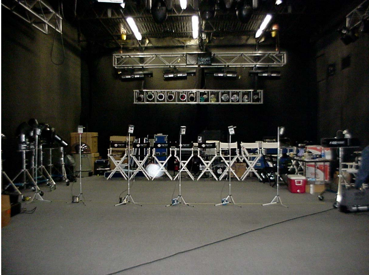
Figure 2. Sampling configuration consisting of six sampling/monitoring tripods situated at three foot intervals from a smoke or haze machine (far right). Each tripod is equipped with an aerosol monitor. The tripods situated at distances of 6, 9, 12, and 15 feet are also equipped with sampling pumps, flexible tubing, and collection media.
